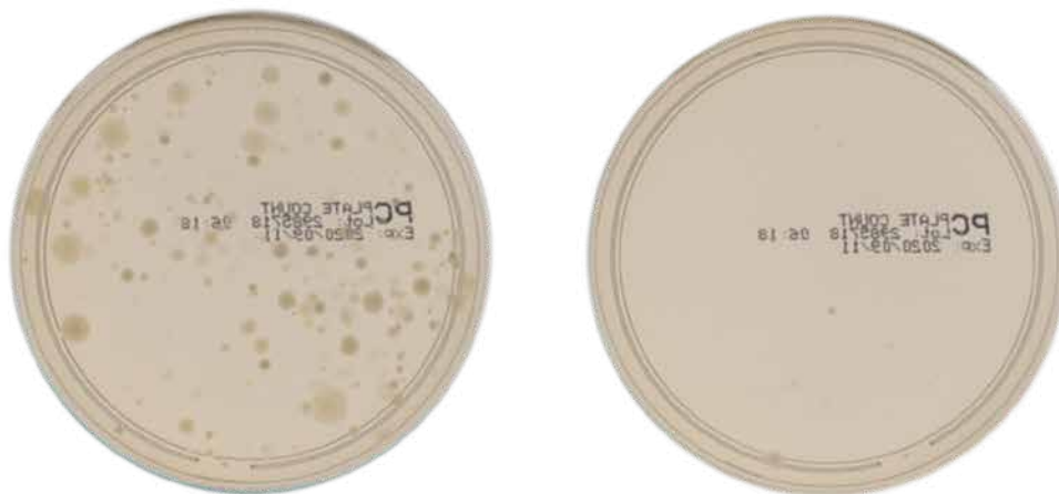
Total number of germ colonies (dark spots) in the untreated sample from the clear water phase in the secondary clarifier (left) and in the treated sample (right).
