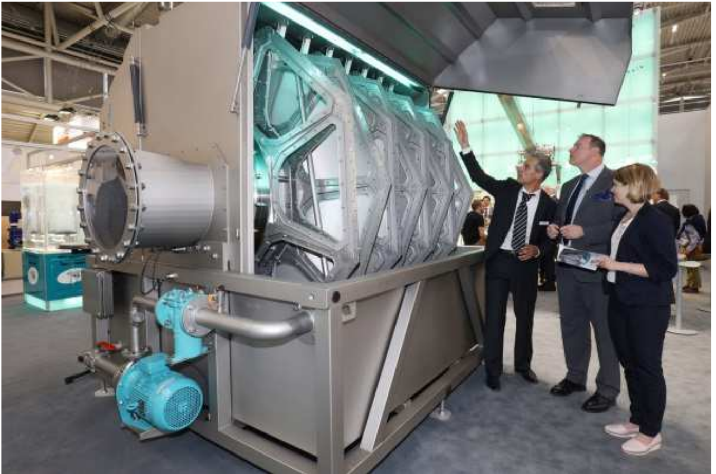
Pic. 1: INVENT iFILT ® - Diamond Filter with six filter disks
