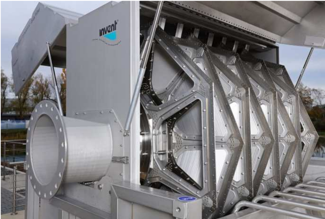
Pic. 3: A look inside the iFILT®-Diamond Filter
